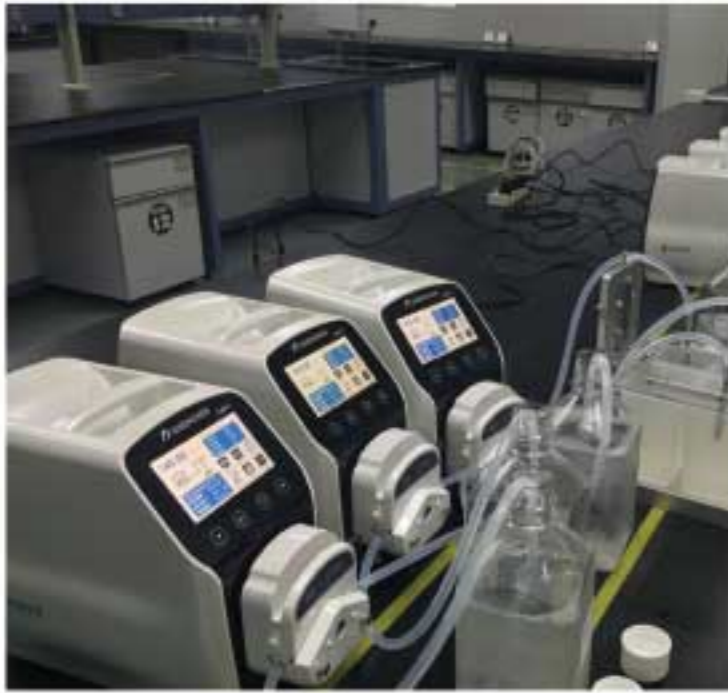
Laboratory chemical dosing
