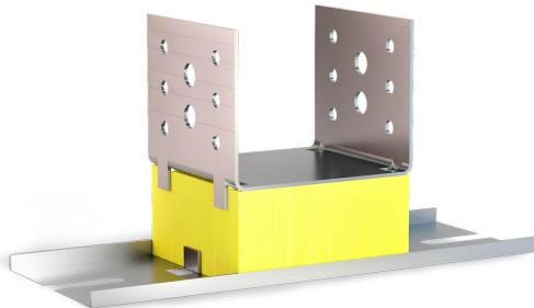
Akustik+Sylomer® Floor Mounts have been conceived for the suspension of floating floors. The excellent properties of the Sylomer® microcelular polyurethane achieve elevated isolation values as opposed to other mounts using rubber or cork, or a combination of both.
