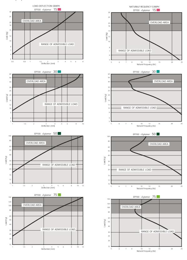
Rubber Metal anti vibration mounts
