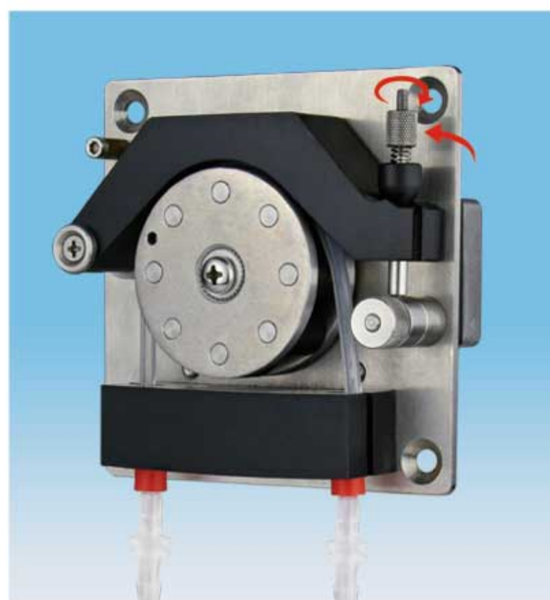
4. Turn spanner anticlockwise, locking the upper block, micro adjust the occlusion.
