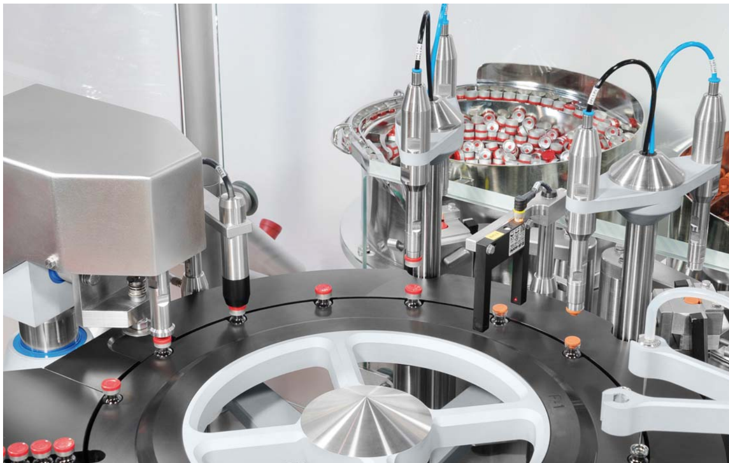
Transport system of vials adapted to laminar flow conditions.
