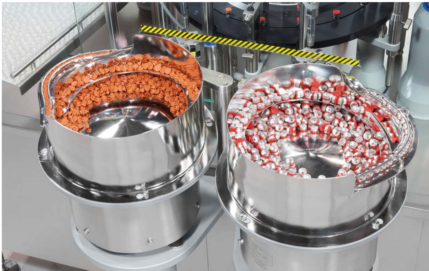
Feeding of stoppers and caps is done automatically through vibrating feeders made of AISI-316L stainless steel.
