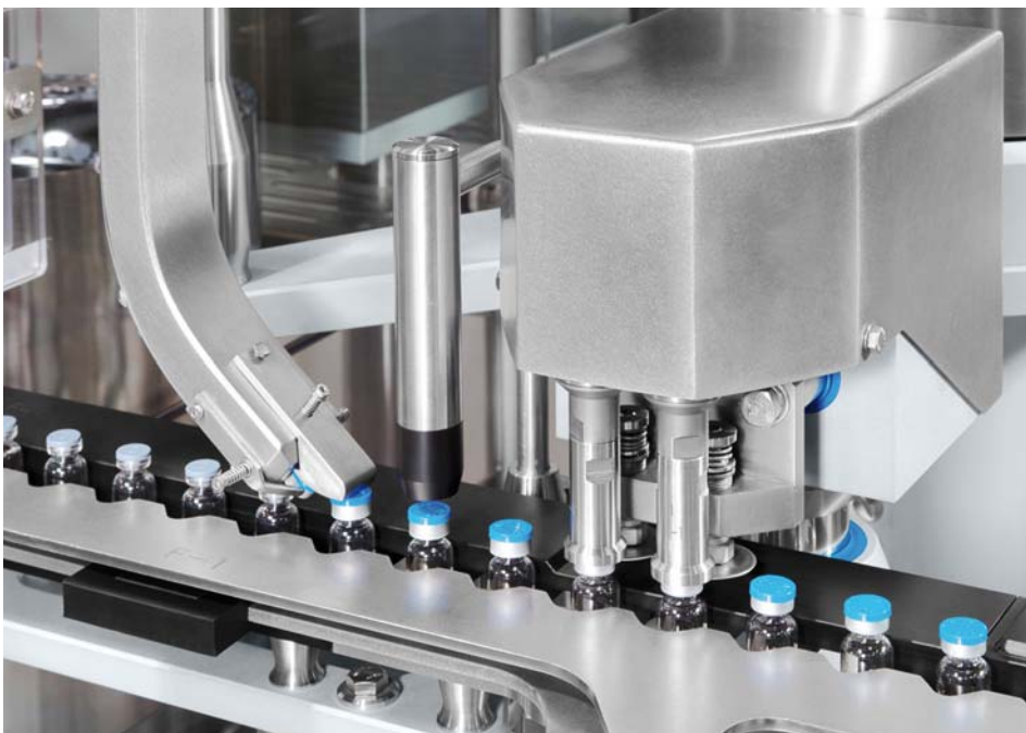
The closing station is equipped with a tangential rolling head, characterized by a minimum generation of particles during the closing process.
