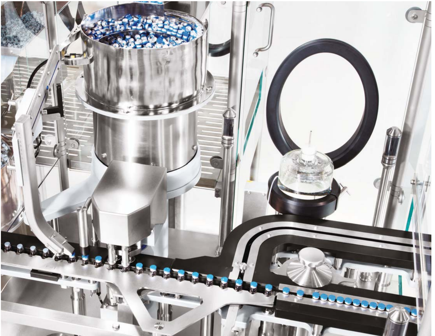
Aluminum cap positioning, closing station and rejection of vials with process defects.
