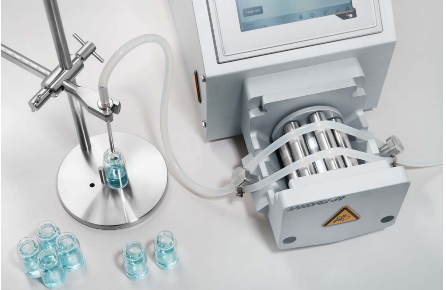
Peristaltic head with 6 or 8 rollers, made of AISI-316L stainless steel, and two separated tracks for accurate and pulse-free pumping.
