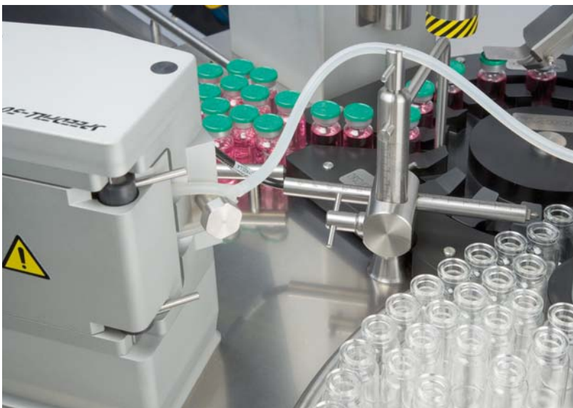
A SpeedFill ® pump integrated into a filling and closing monoblock of intermittent motion.
