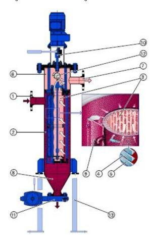
The filtered fluid exits the filter housing at the top opposite the inlet connection. In the AF 94 S version, the integrated preseparator relieves the filter cartridge of coarse and heavy particles by means of a tangential flow around the tube.
