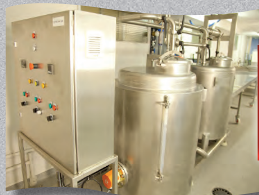
Cleaning station using reverse osmosis water
