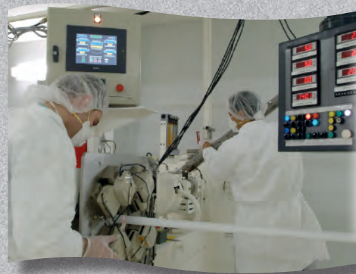
Our cleanroom: 700m 2 in a controlled atmosphere area for the silicone hoses production
