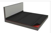
7) (Optional) Install PE-foil (0.2 mm). Overlap joints about 20 cm. Top edge of the PE foil 15-20 cm above finished floor level.
