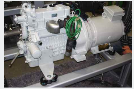
Small combined heat and power plant
