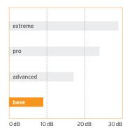
Experimental set-up: 50 kg – 50 cm drop height 18 mm sports floor (16 kg/m²) 12.5 mm Shock Absorb base (2.5 kg/m²) 140 mm reinforced concrete ceiling (350 kg/m²)
