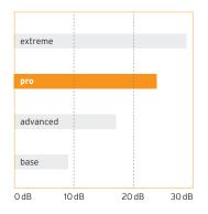
Experimental set-up: 50 kg – 50 cm drop height 18 mm sports floor (16 kg/m²) 50 mm Shock Absorb pro (10.13 kg/m²) 140 mm reinforced concrete ceiling (350 kg/m²)
