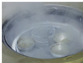
Shock freezing of plant pollen in a laboratory freeze-dryer with LN 2
