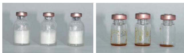
Figure 4.14 Properly dried product (left) and melted, splattered product (right)
