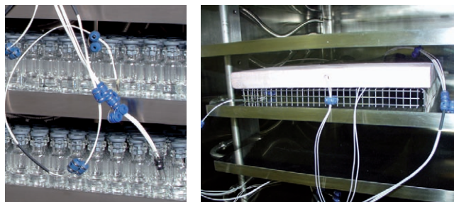
Figure 5.4 Product sensors in a 1 cm high beaded-rim flask filled with an active substance and in a spongy product
