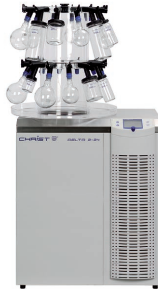
Figure 3.1 Freeze dryer with acrylic glass drying chamber (a) and rubber valves (f)
