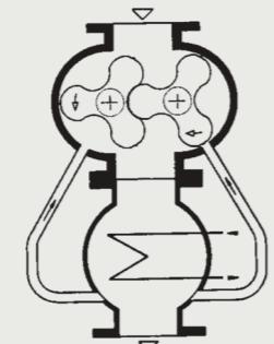
If it is necessary to recover or re-compress the pumped gas, the cooling gas must be taken in from a gas cooler arranged in series connection (Fig. 2).
