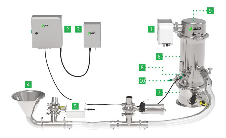
**piFLOW**°**p SMART is a complete system.** It has a heart, a brain and senses. At its heart (1), vacuum is created with compressed air and Piab's COAX° technology. The system's brain, the Electrical Control Unit (2), automatically controls the pump. It does so with the help of its Valve Unit (3) where vacuum and pressure are being sensed, and electrical signals converted into pneumatic ones.
