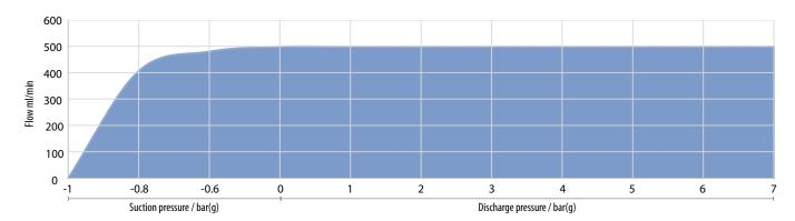
Flows are typical and were measured with water at 20°C. Actual flows will vary according to suction conditions, discharge pressure and normal component production tolerances.
