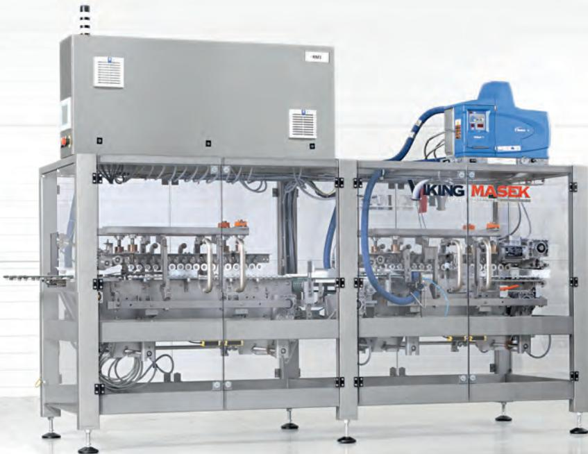
Viking Masek's CLM machines are a family of carton closing machines. We offer straight-line or right-angle units to close one, two or three flaps of the cartons.
