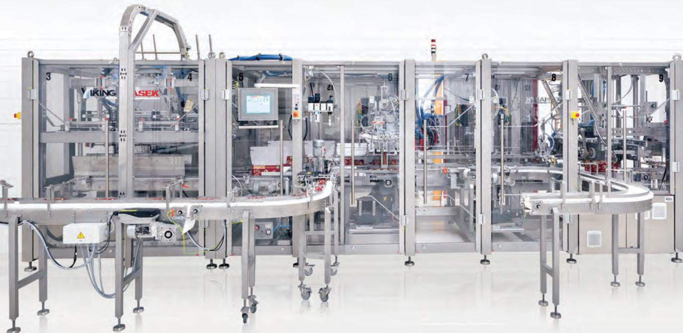
It is often said that life is a series of trade-offs. But not for Viking Masek's unique top load solution MFM – multifunctional machine combining carton erector, product loading unit and carton closing machine into one compact unit. The MFM has the unique capability of being able to match available floor space.
